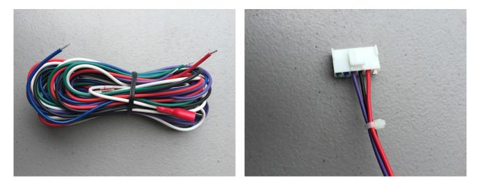
Unit comes with 6 wires in the harness You will only need these 3 wires (Red, black, purple) Electrical Connections: Make ALL electrical connections prior to plugging the main wiring harness into the base unit.
